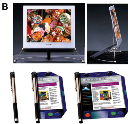
(B) Organic light emitting diodes can be used to make thin and flexible displays. Adapted by permission from Nature, Forrest [2].
