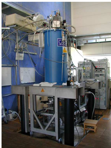
(a) Overall view: the cryostat and the air legs are visible
