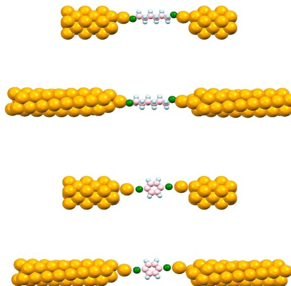
**Figure 1.** Relaxed junction geometries of hexanedithiolate bonded to gold adatoms on Au(100) and Au(5,3) electrodes and of benzenedithiolate bonded to gold adatoms on Au(100) and Au(5,3) electrodes (from top to bottom, respectively), along the  $z$  axis and lying on the plane which is  $45^\circ$  to the  $yz$  plane.
