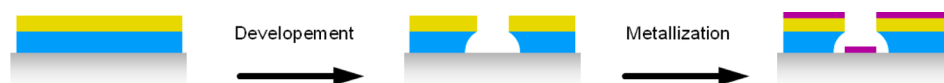
Figure 2. Illustration of the process steps used for patterning nanoelectrodes by EBL with SiO 2 (300 nm; gray), PMGI (45 nm, blue), PMMA 950 K (25 nm, yellow), and platinum (13 nm, violet).
