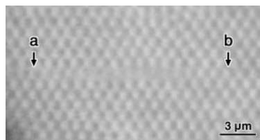
Fig. 4. Disappearing images of more vortices in a single chain ( T = 57 K, B_{\perp} = 0.8 mT, \theta = 80^{\circ} ). We attribute the disappearance of the vortex images to the synchronous oscillation of vortices between the node vortices a and b along the chain direction, just like a coupled oscillation.
