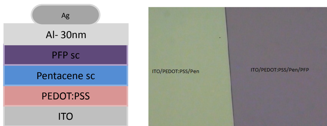
Figure 1: Sample structure (left) and image of PFP single crystal edge on top of the pentacene single crystal (right).
