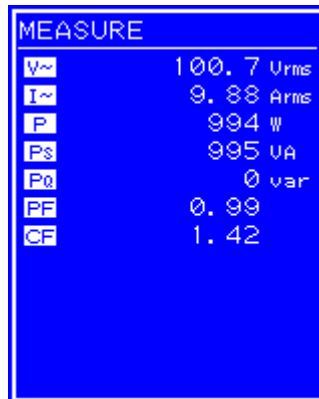
Figure 4-3. Example of Measured Value Window (During AC+DC Mode)
