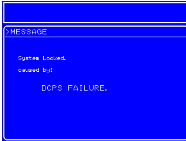
Figure 7-2. Screen Display When Protection Function-Related Error Has Occurred
