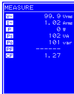
Figure 3-12. Example of Measured Value Window (AC-INT Mode)
